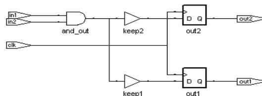
Without `syn_keep` out1 and out2 optimize into one register.
