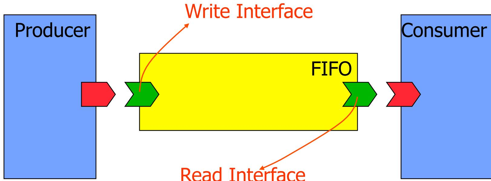
**Problem definition:** FIFO communication channel with blocking read and write operations
