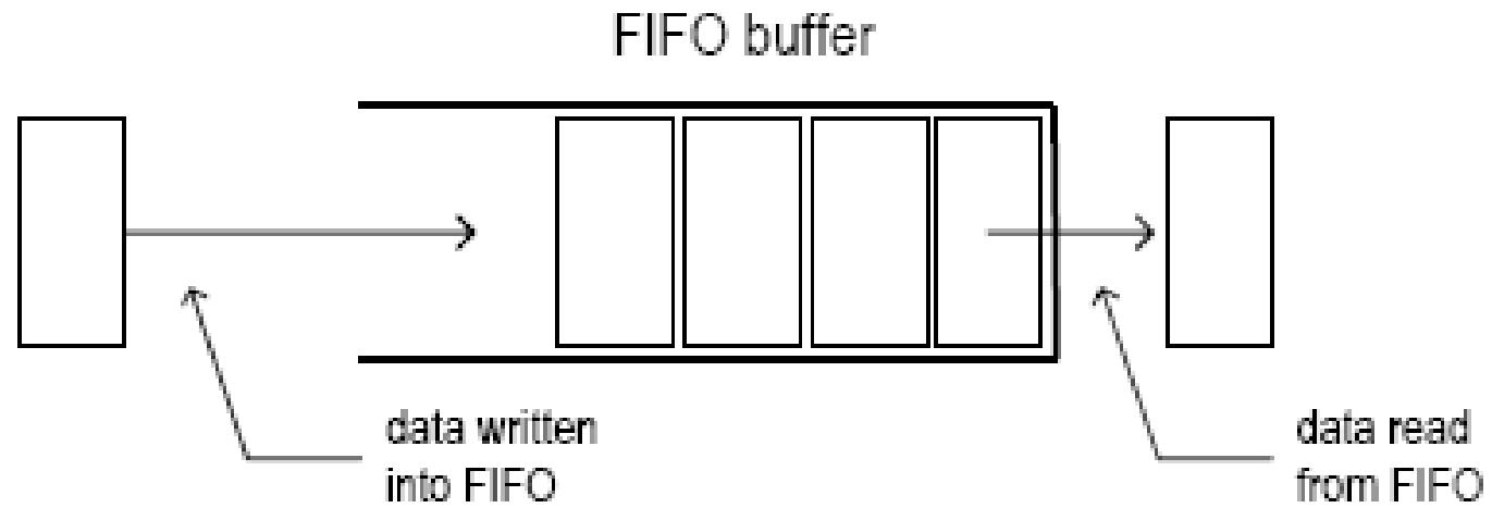
**Figure 9.11** Conceptual diagram of a FIFO buffer.
