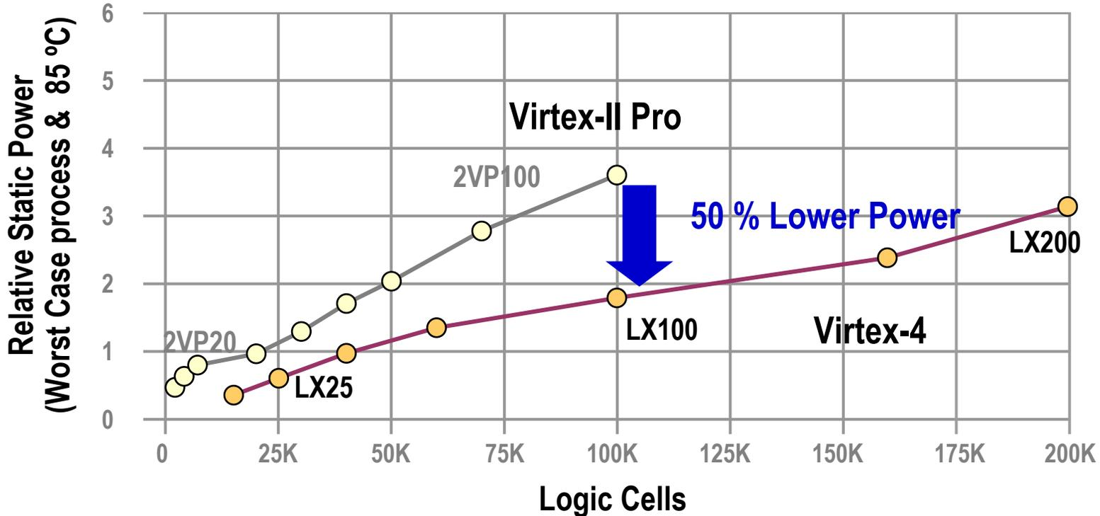
**Virtex-4 has 50% lower static power than Virtex-II Pro**
