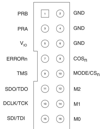
Figure 1-1. Silicon Explorer II Probe Connector Pin-Out
