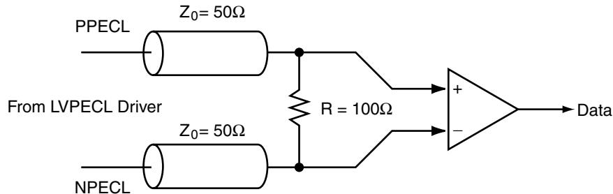
**Figure 9 • Recommended Termination for LVPECL Inputs****Table 4 • LVPECL Receiver Specifications**
