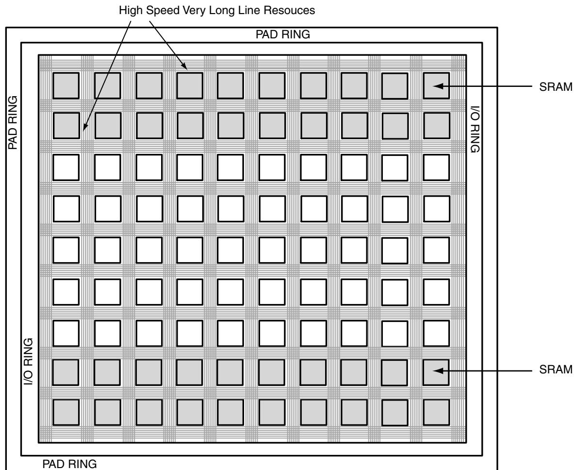
**Figure 6 • High Speed Very Long Line Resources**
