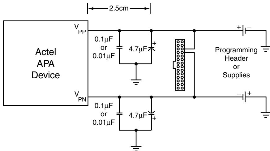
**Figure 21 • ProASIC<sup>PLUS</sup> V<sub>PP</sub> and V<sub>PN</sub> Capacitor Requirements**
