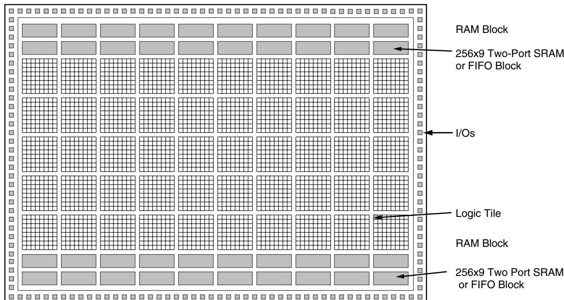
**Figure 1 • The ProASIC<sup>PLUS</sup> Device Architecture**
