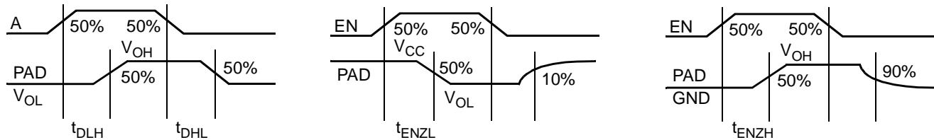
**Tristate Buffer Delays**(Worst-Case Commercial Conditions, V<sub>DDP</sub> = 3.0V, V<sub>DD</sub> = 2.3V, 35 pF load, T<sub>J</sub> = 70°C)
