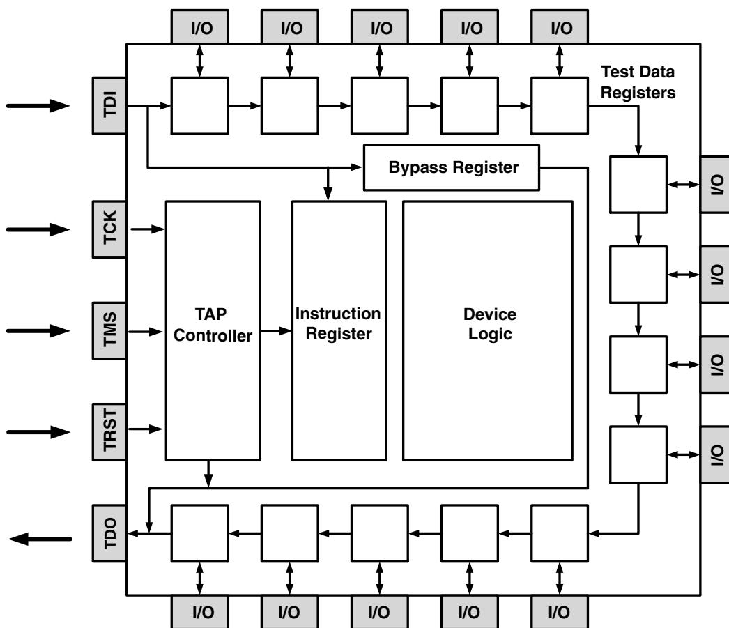
Figure 10 • ProASIC<sup>PLUS</sup> JTAG Boundary Scan Test Logic Circuit
