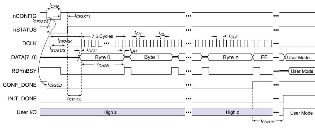
Tables 14 and 15 define the timing parameters for PPS configuration in APEX 20K and FLEX 10K devices.
