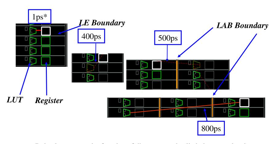
Delay is not a regular function of distance at a detailed placement level
