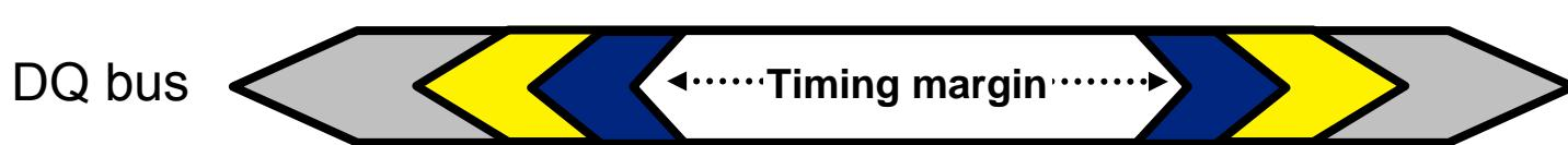
Timing margin based on dynamic calibration
