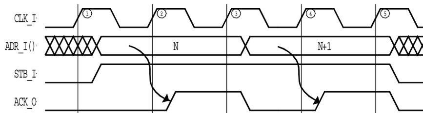
Figure 4-3 WISHBONE Classic synchronous cycle terminated burst
