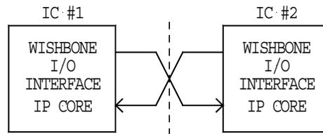
Figure 1-6. Off-chip interconnection.
