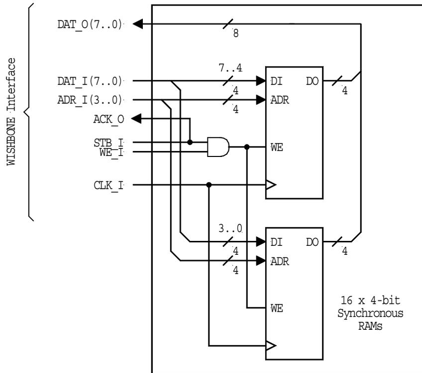
Figure A-16. Simple 16 x 8-bit SLAVE memory.
