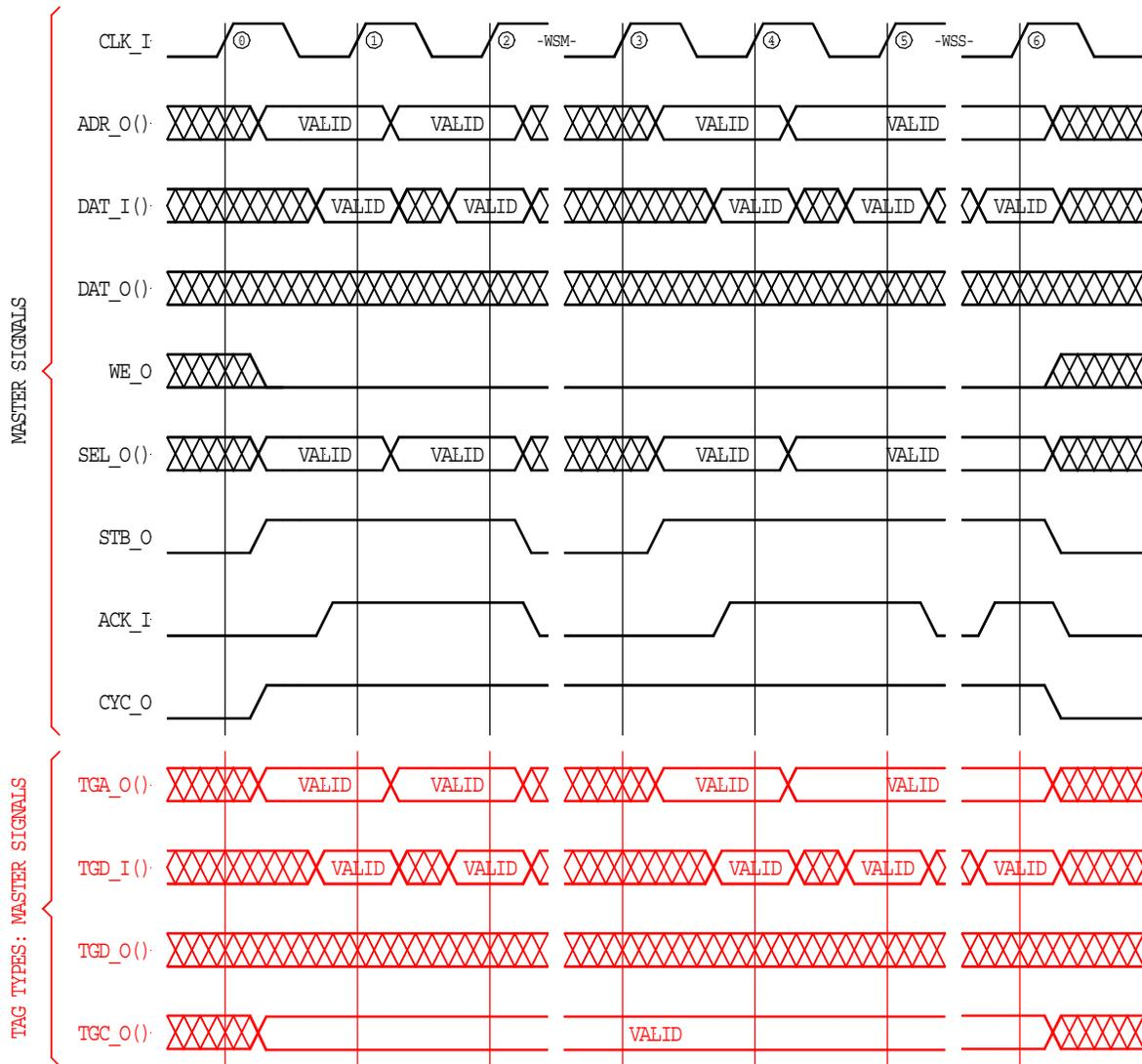
Figure 3-6. BLOCK READ cycle.
