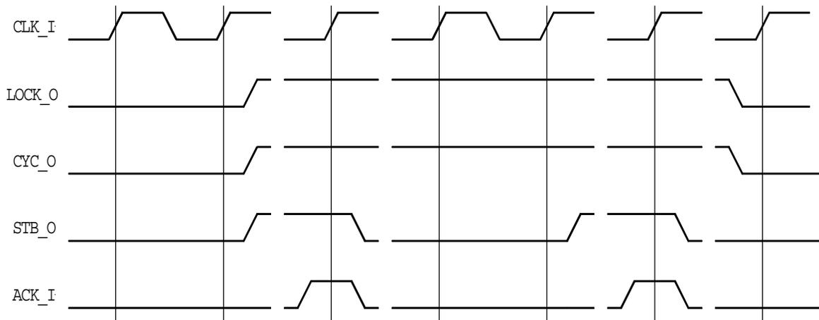
Figure 3-5. Use of [CYC\_O] signal during BLOCK cycles.
