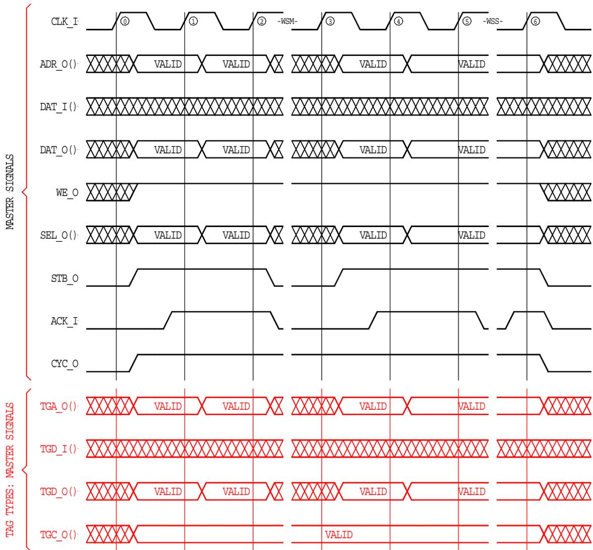
Figure 3-7. BLOCK WRITE cycle.
