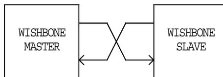
Figure A-2. The point-to-point interconnection.
