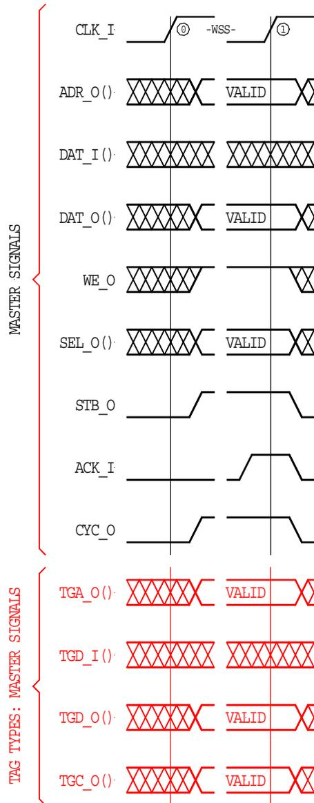
Figure 3-4. SINGLE WRITE cycle.
