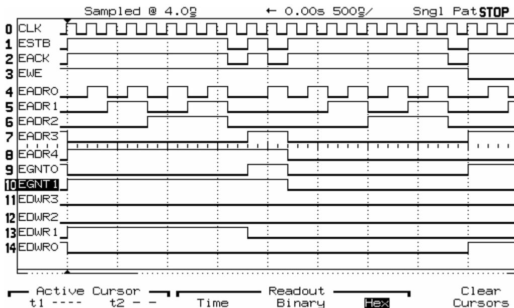
Figure A-27. Logic analyzer trace on the Spartan 2 evaluation board<sup>16</sup>.
