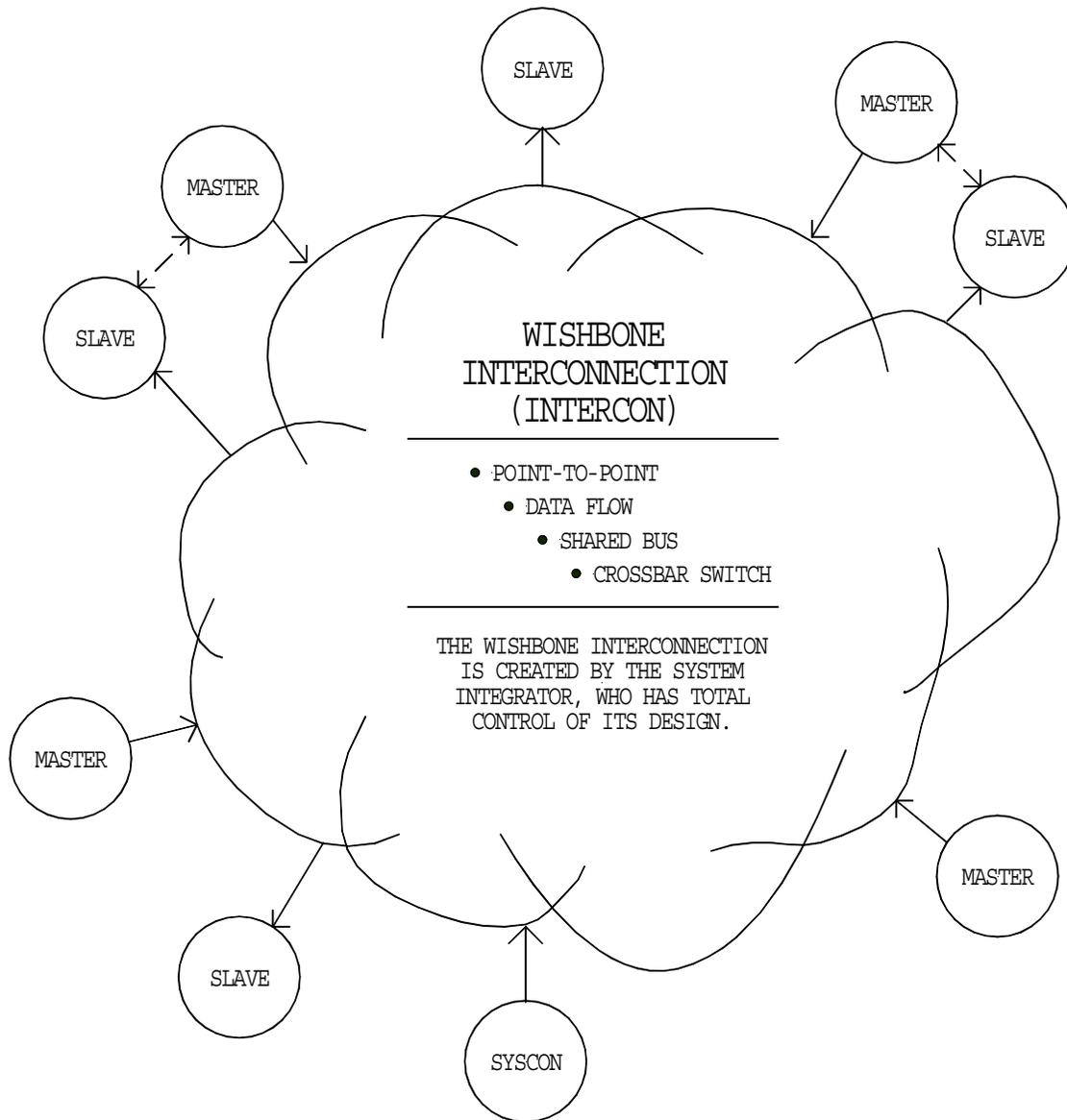
Figure A-1. The WISHBONE interconnection.
