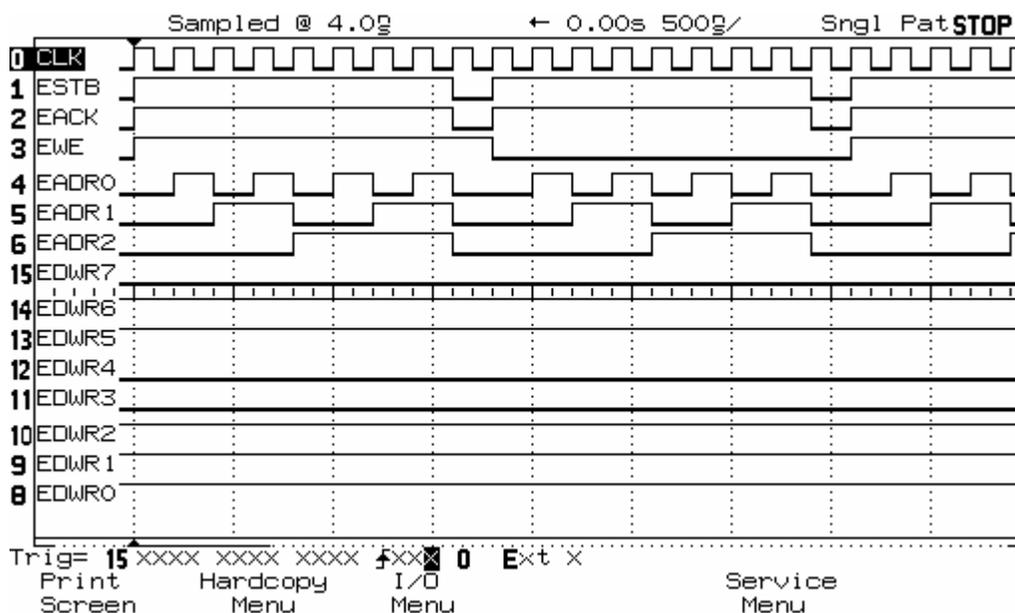
Figure A-18. Logic analyzer trace on the Spartan 2 evaluation board<sup>11</sup>.
