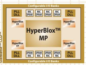
programming the HyperBlox FP fabric. Like any other SRAM-based FPGA, this fabric allows for an unlimited number of reconfigurations by simply downloading a new bistream into the device, thus offering optimal in-field programmability.
