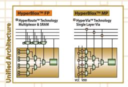
The HyperBlox MP fabric uses the same logic core cell architecture as HyperBlox FP but replaces the SRAM configuration with a single-layer via-mask configuration, called HyperVia<sup>TM</sup>.
