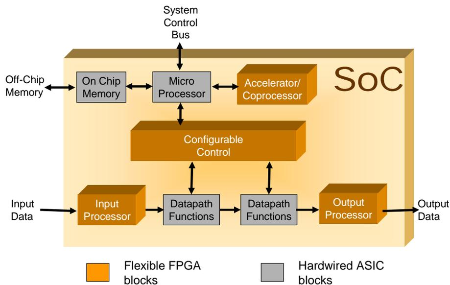
Figure 2. Partitioning between hardwired and flexible functions
